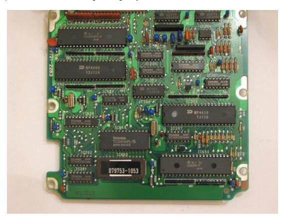
We need to remove IC660 (the chip with the stick on label at the bottom left of the above picture, closeup pic below). The board will also be silk screened with IC660.
