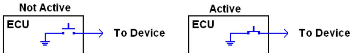
While the diagram above depicts a switch in the ECU for simplicity, the actual switching circuit utilizes solid state components. These components have a much lower current limit than a switch or relay. If you must control a device that can draw more than 500ma of current, you must use a relay
