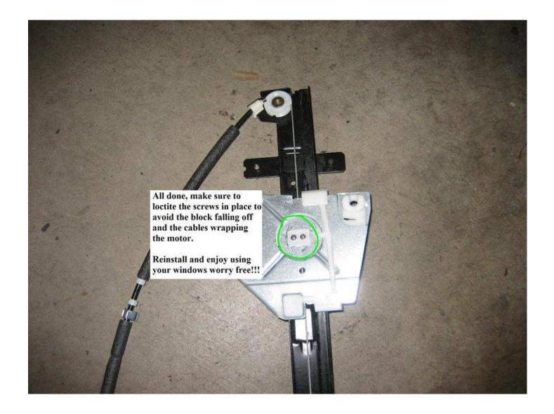
18. Reverse the process and reinstall the regulator - Now you can use the windows without worrying about that impending "BANG" you'll hear as you watch the glass disappear into the door....
